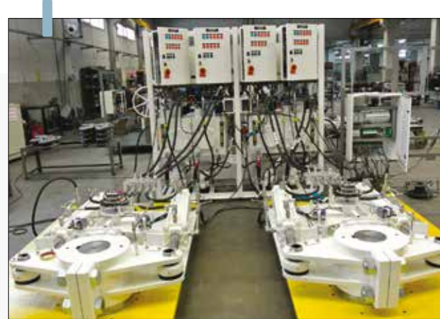
DDS 8000x2 Electronic synchronised steering gears under test at factory
