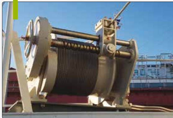
Hydraulic hoisting winch with spooling
