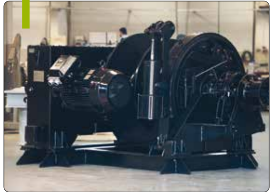
Electric motor driven combined fore towing winch
