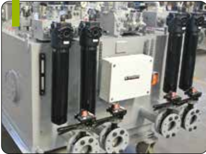
Main engine driven power unit hydraulic tank.
