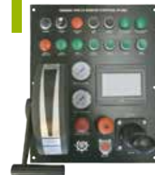
Towing winch control panel with display unit.
